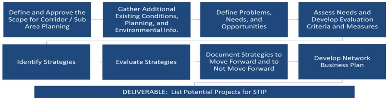
Figure 2. Phase 2 Steps of the UDOT Corridor Planning Process.
