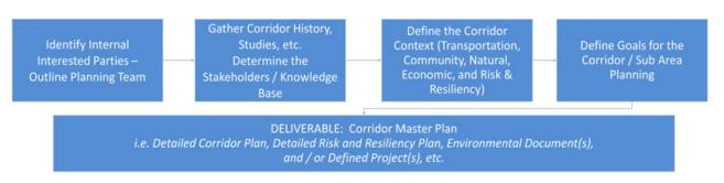
Figure 1. Phase 1 Steps in UDOT Corridor Planning Process (UDOT, Available at: http://gis.bio-west.com/corridorplanning)
