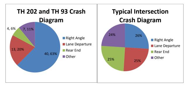
Comparing this intersection to other intersections in Minnesota, it appears that right angle crashes are over represented at TH 202 and TH 93. When possible, obtaining intersection collision diagrams can also be insightful into understanding the problem.
