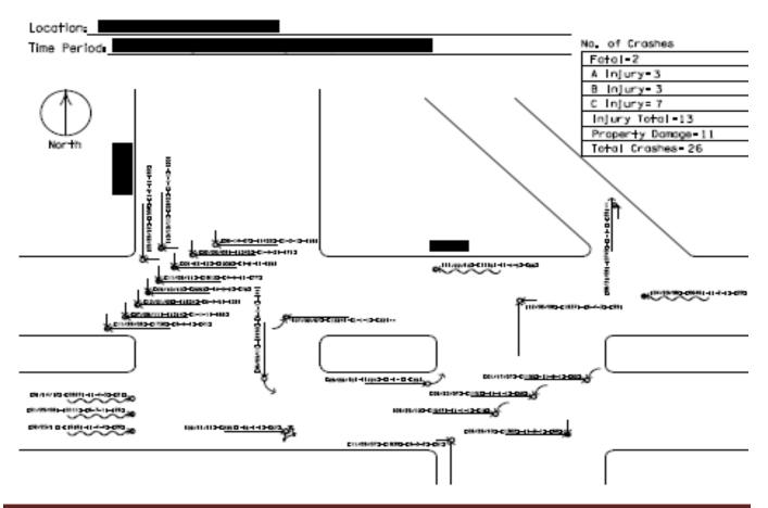
The collision diagram for this intersection shows a large number of crashes (and especially severe crashes) are occurring on the near side of the intersection. If the goal is to make this intersection safer, this crash type should be our target to eliminate.
